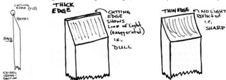
Edge tools ought to be sold sharp, but they rarely if ever are today. It is not practical to reduce substantial thickness by honing (rubbing on a whetstone). In the Western tradition, grinding (on the edge surface of a rotating abrasive wheel) does this. This is fast and effective. However, grinding to sharpness does not produce an edge that is ready to use. A ground edge has two flaws that must be removed by honing: 1. Coarse edge texture. 2. Burr. And there are
