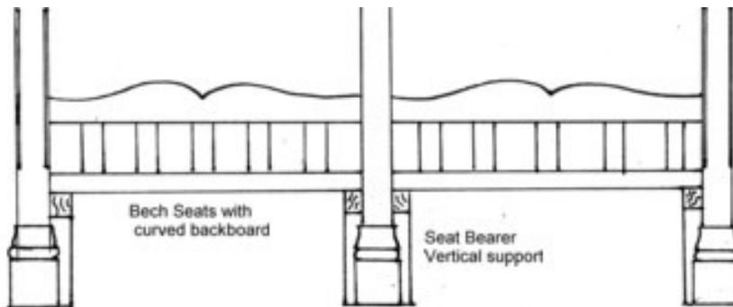
The backboard is cut using a jigsaw to any shape you prefer. Pictured is the standard moulding seen on these pavilions. Pickets are then cut and dowelled between the curved topboard and the bottom seat.
