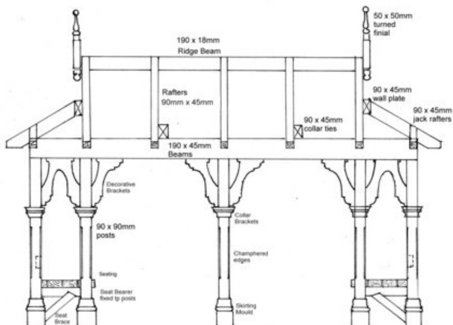
The rafter spacings can be set out on the beam and the ridge and the remaining long rafters fitted and nailed. Two braces are required at a 45 degree angle across the top of
