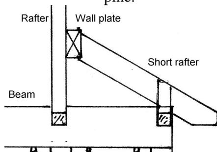
A small hip rafter is cut to sit on 45 degrees to the rafters, and is to be birdsmouthed to the same height as the rafters. Nail these hips to the wall plate and rafter.
