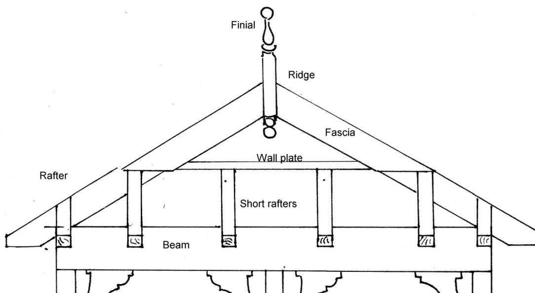
Measure the small rafters using the method described in step 4, including the same birdsmouth, and angle at the top (plumb cut). Install the rafters starting with one on either end of the plate and position flush with the top of the longer rafters. These can be skew nailed into the plate.
