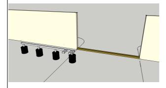
3 Install the baseplate so the top face is flush the top of the driveway slab.
