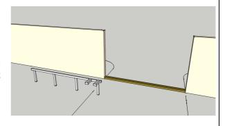
**5**Excavate and install the top roller support post (if required)
